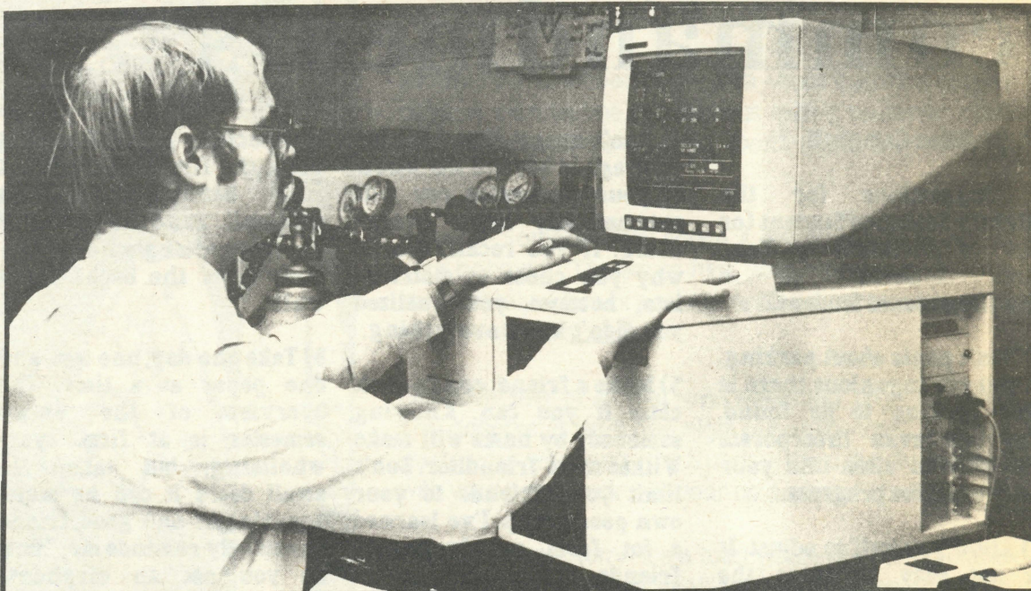
Dr. Mike Case tests an environmental sample on the Water Quality Testing Lab's new gas chromatograph, which is controlled by a microprocessor.
